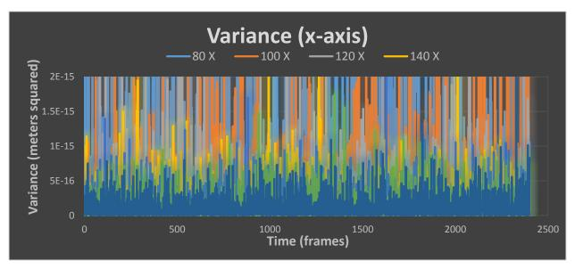
The legend in this graph describes the laser power in milliwatts. As the power is increased, the variance decreases. Our CCD camera was capturing 409 frames per second. You can see that the particle's Brownian motion was decreasing.
