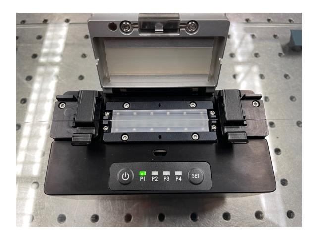
Press the "SET" button and wait for the flashing green lights to turn solid. The cure will be complete after one cycle. Open the safety cover of the ProCoater and release the fiber clamps. The fiber will be wedged in the mold so carefully remove the fiber by pulling **BOTH** ends of the fiber vertically.
