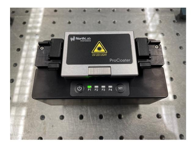
After removal of the fiber, clean the mold delicately by using a delicate wipe and some Isopropyl alcohol. Close the safety lid of the ProCoater and turn off the device when done.
