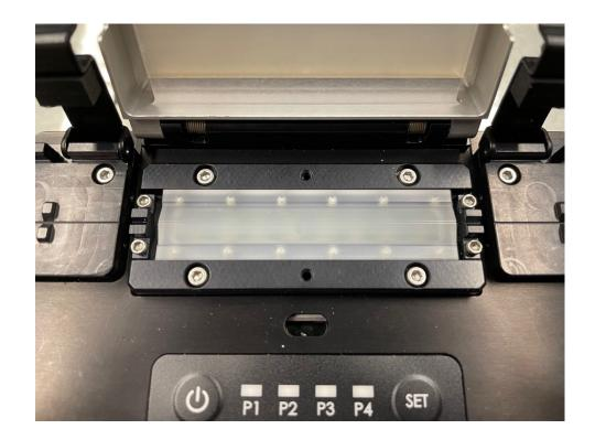
Place the center of the fusion spliced fiber in the center of the mold and secure the fiber down, in the fiber channels, with the fiber clamps.
