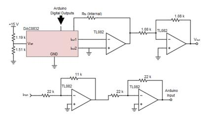
Fig. 7: Arduino Control Circuit Diagram
