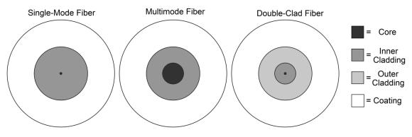
Fig. 4: Double-Clad Fiber
