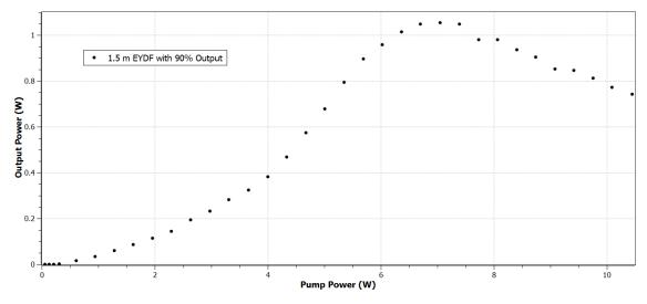
Fig. 10: 1550 nm Output Power vs. Launched 975 nm Pump Power up to 10 W Evolution of the output power as a function of pump power, for 1.5 m of EYDF
