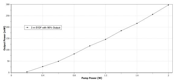
Fig. 11: 1550 nm Output Power vs. Launched 975 nm Pump Power up to 2 W
