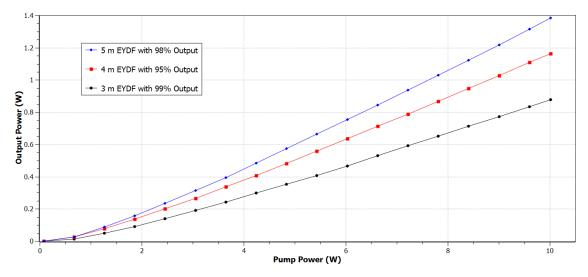
Fig. 14: 1550 nm Output Power vs. Launched 915 nm Pump Power up to 10 W Evolution of the output power as a function of pump power, for 3 m, 4 m, and 5 m of EYDF pumped with 915 nm light.
