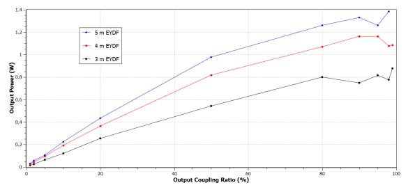
Fig. 16: 1550 nm Output Power vs. Output Coupling Ratio
