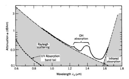
Fig. 5: Attenuation in Silica Fibers
