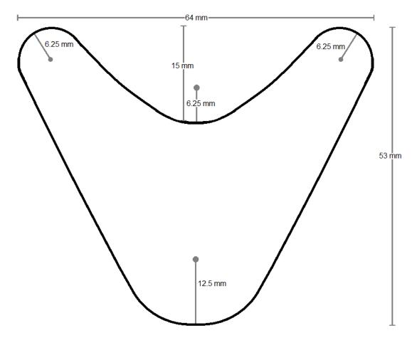
Fig. 13: Optimized Mode Scrambling Geometry
