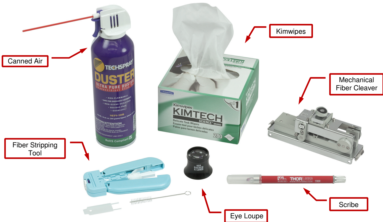
Figure 26 Tools for the manual cleaving of an optical fiber.
