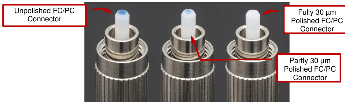
Figure 20 Three FC/PC connectors, from left to right, showing an unpolished, partly polished, and completely polished fiber using the 30 \mu\text{m} polishing film.
