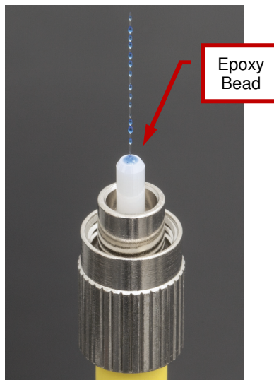
Figure 11 Proper sized epoxy bead on a SM fiber (Item # SMF-28e) and FC/PC connector (Item # 30126C3).
