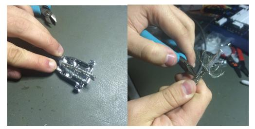
Peel off the remaining metal foil layer to find the multi-colored wires. Add around 5 mm of heat-shrink tubing to each of the wires (the picture shows too much heat-shrink tubing). Next, strip off the tip of each colored wire's plastic wrap so that the wire can be soldered.
